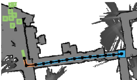
(e) The third SDC (“go straight to the cabinet”) contains some information about the location of the cabinet (it is straight ahead). The policy generates a landmark distribution for its location.
