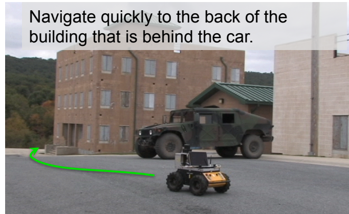
Figure 8.1: The Husky robot platform executing a natural language command in an outdoor environment.
