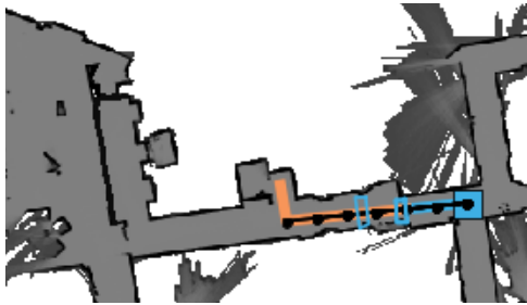
(c) When a right turn is available, the policy decides to take it even though it leads into a bathroom.
