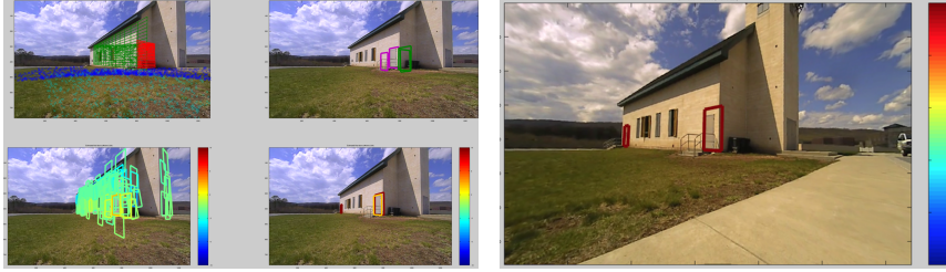
Fig. 5: Examples of door detections are shown. Façade detection and door candidates are shown on the left. Final detection output is shown on the right.
