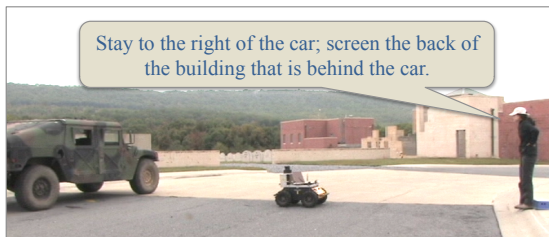
Fig. 1: An example showing a Clearpath TM Husky unmanned ground vehicle working with a human teammate on a screening mission in an unknown environment.
