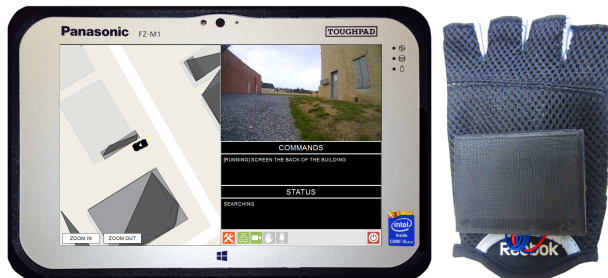
Fig. 3: An illustration of the Multi-Modal Interface (MMI) for human-robot interaction. The MMI accepts input in the form of speech and/or gesture and visualizes the state of the intelligence architecture. The MMI Visual Display illustrates a “screen the back of the building” command. The robot status shown in the COMMANDS and STATUS sections indicate the command is still running and the robot is currently searching.
