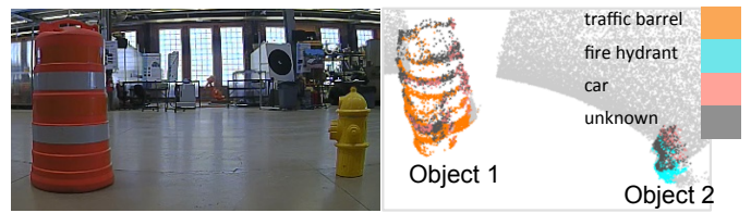
Fig. 6: The 3D classification: Both Object 1 (traffic barrel) and Object 2 (fire hydrant) are classified correctly with high confidence despite the fact that nearly a half of data points are mislabeled.
